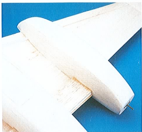
DH Mosquito: Fit the elevators and their adjoining torque rod before adding the tail cone.
