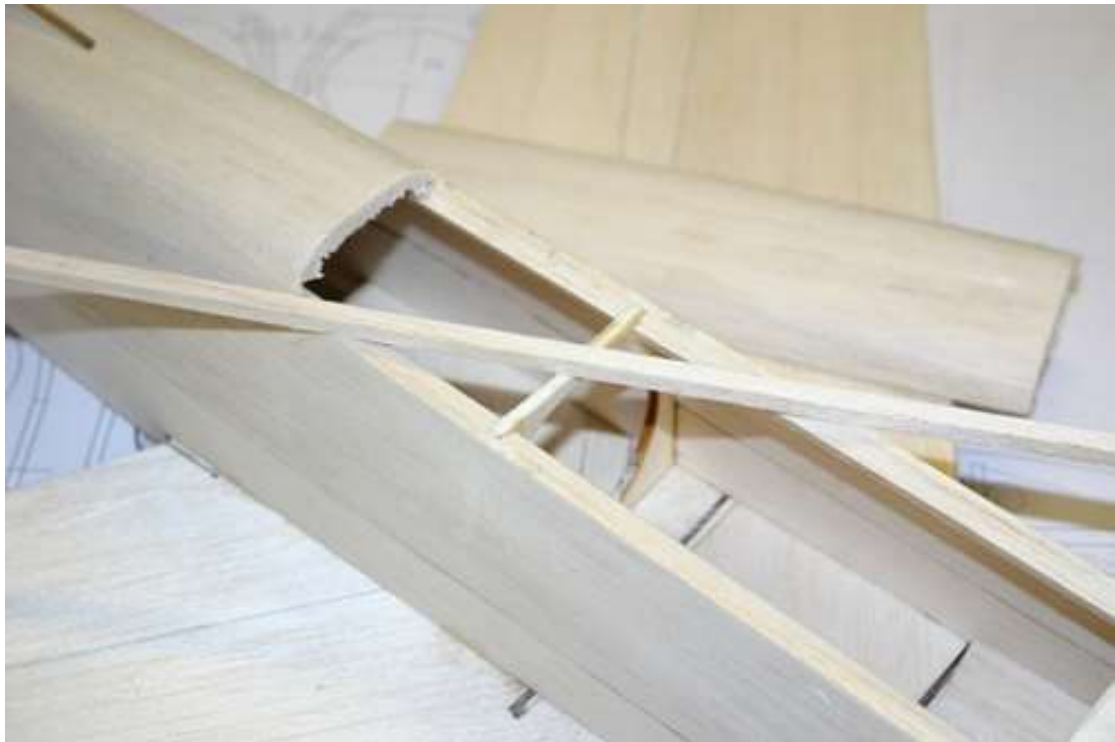
Line the hatch with 4.5mm sq balsa made from scrap
