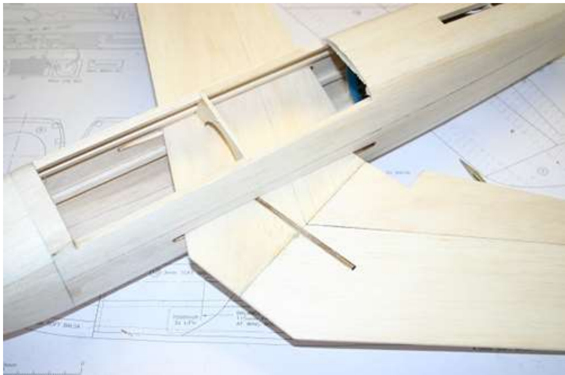
Remove the centre part of from 6 to allow the wings to slide through
