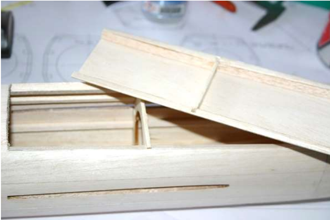
Line the hatch opening with 4.5mm sq balsa made from scrap
