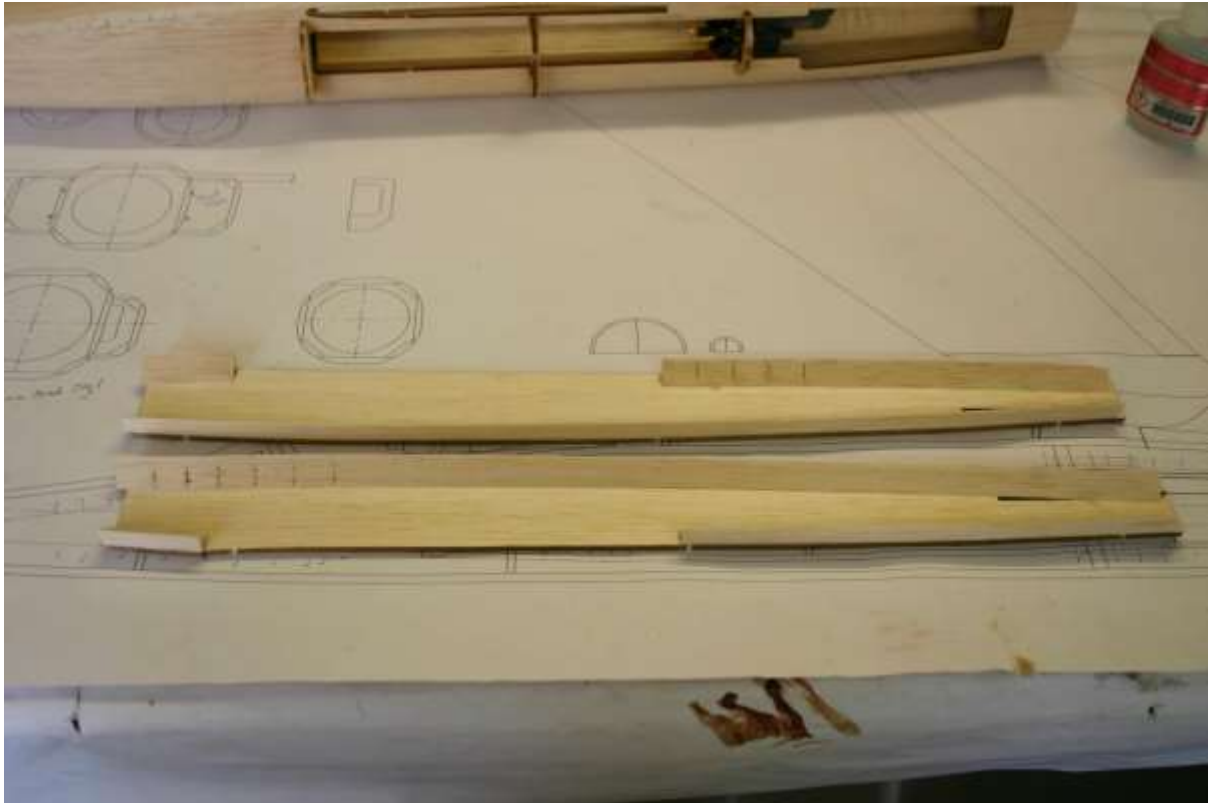
Make up the left and right hand outer fuselage sides
