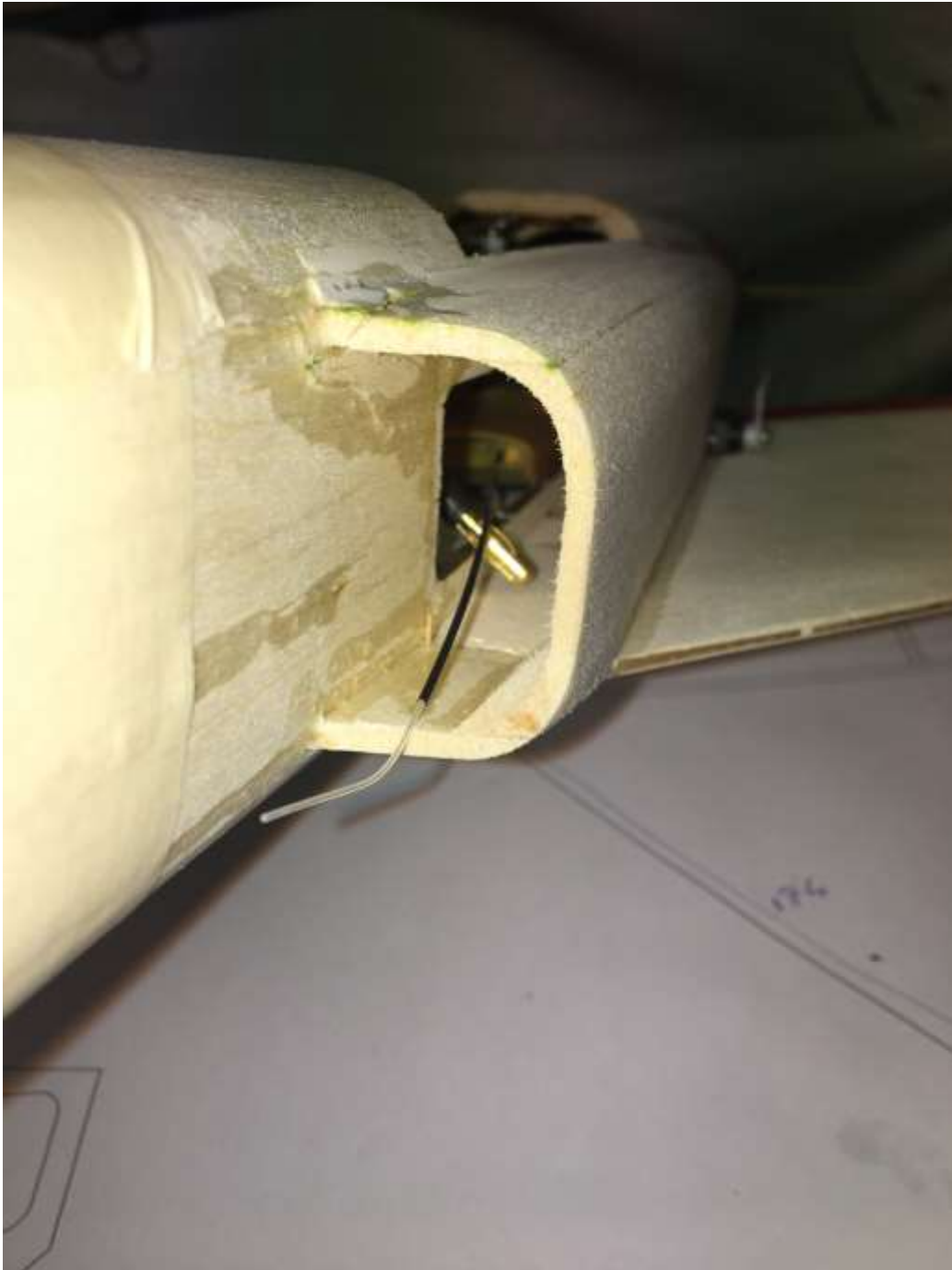
Round off internal triangle to give smooth intake profile
