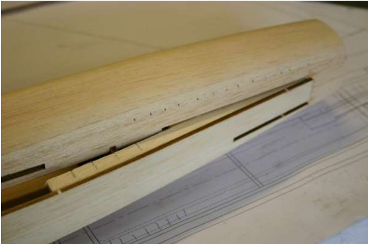
Outer sides 'sink' in to the inner sides at the rear
