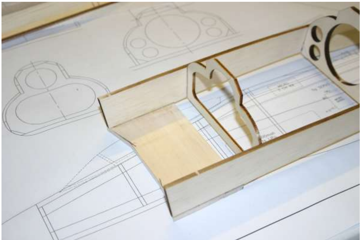
Cross sheet the bottom fuselage just in front of the wing leading edge
