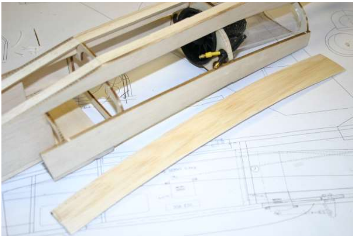
Using the template on the plan and soft wetted 1.6mm balsa, sheet the fuselage sides
