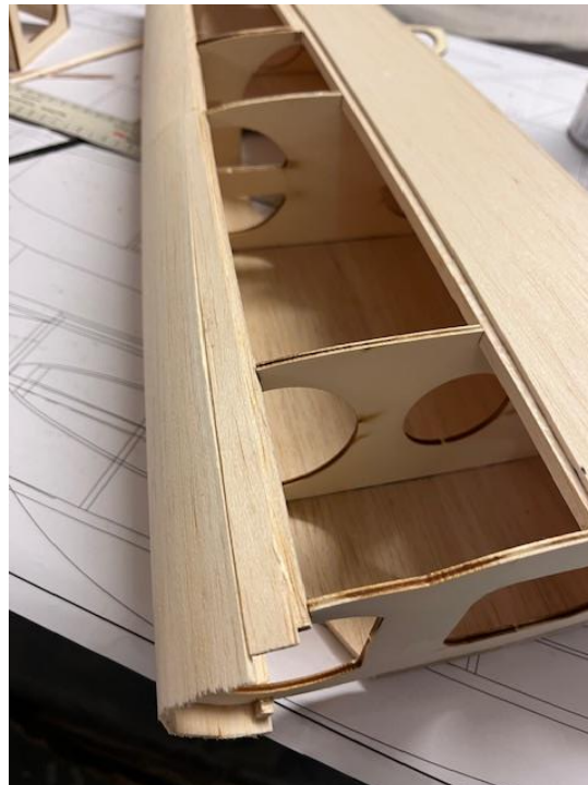
Sheet the side and top. Wet the outside of the balsa to aid bending
