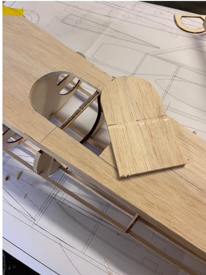
Mark and cut out the fan access, removing the cross bar
