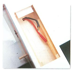
Battery access need not be a problem on the Aerovan, thanks to a handy underside hatch.
