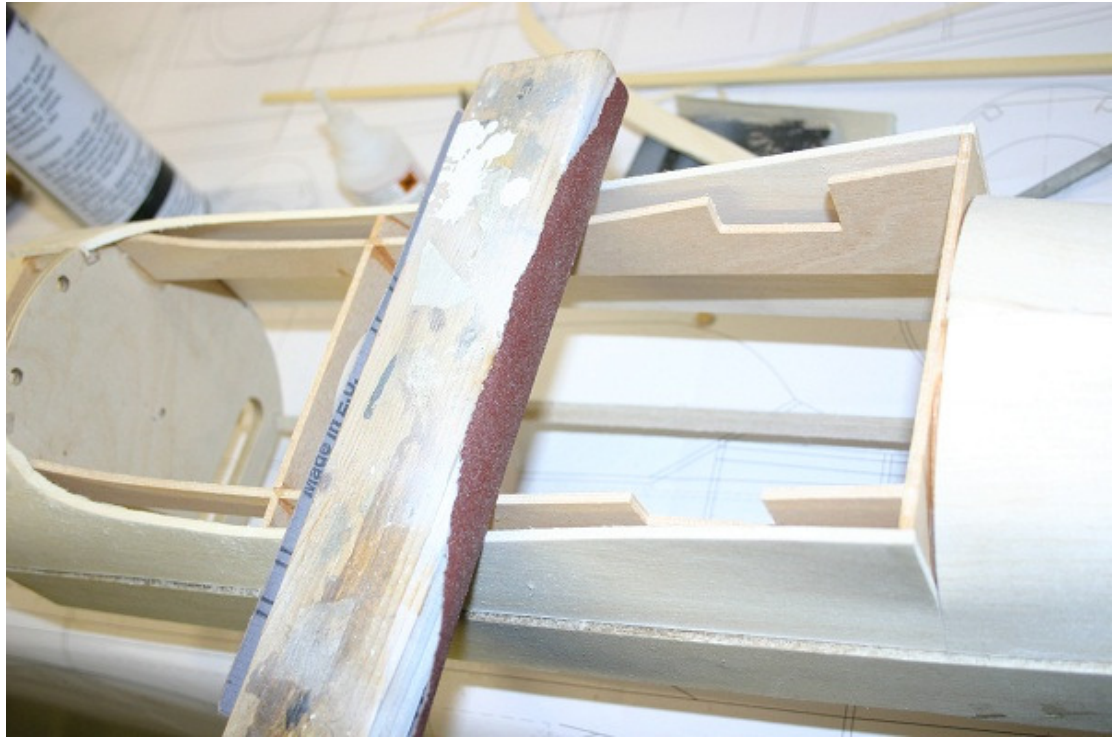
Sanding block to achieve the wing profile
