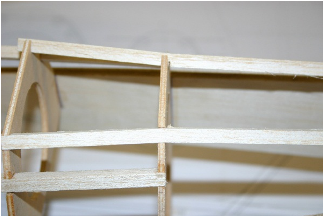
Top stringers cut then bent to shape
