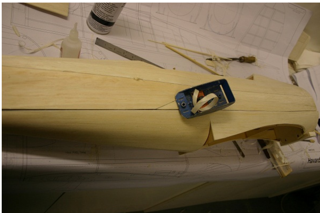
Use razor plane to blend centre section into top & bottom sheeting
