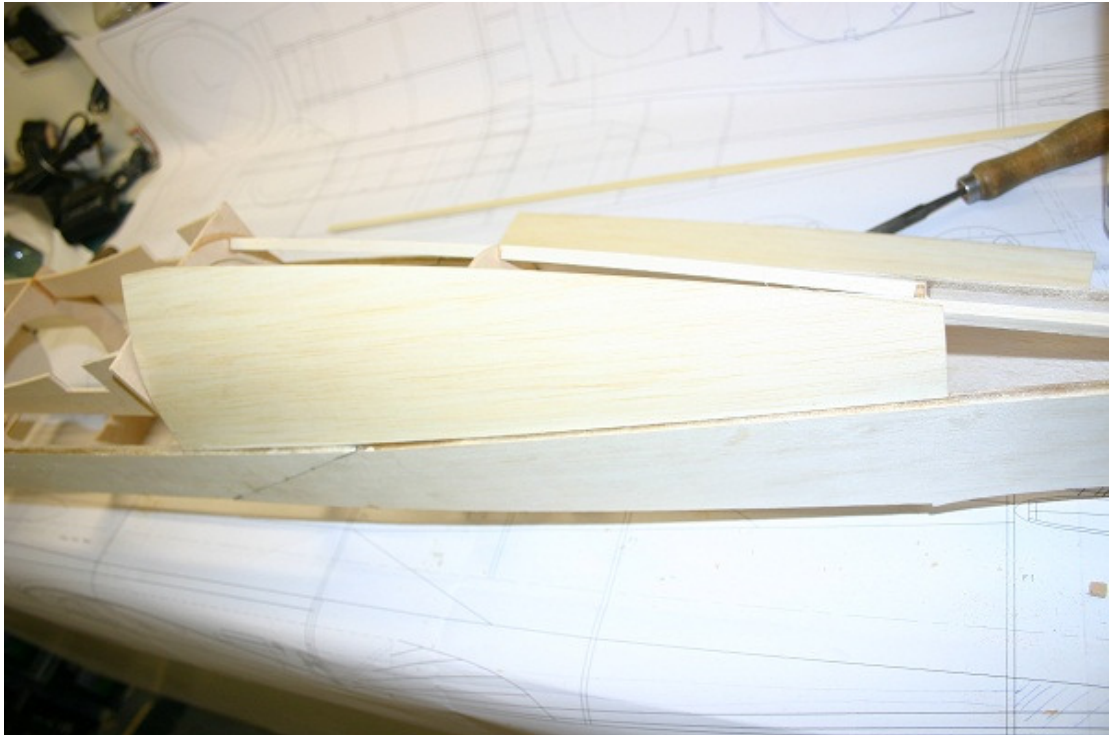
Wet the sheeting to aid bending of lower fuselage sides
