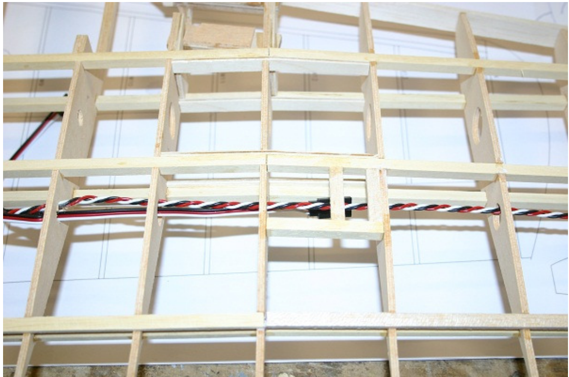
The flap servo mounting points
