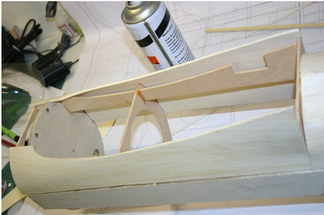
Sheet the forward lower section
