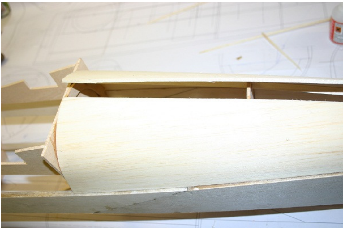
Wet the sheeting to aid bending of lower fuselage sides
