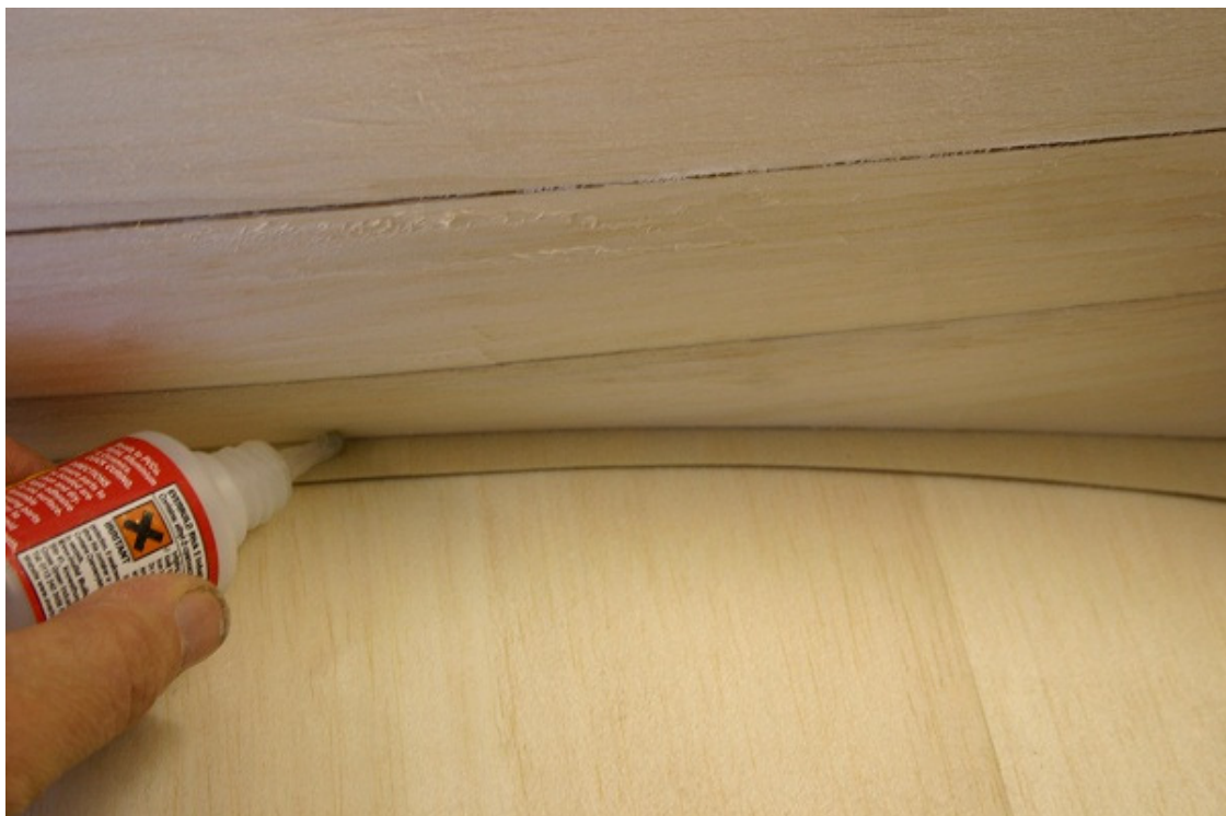
Wing fitted to clap fairing, and then glued
