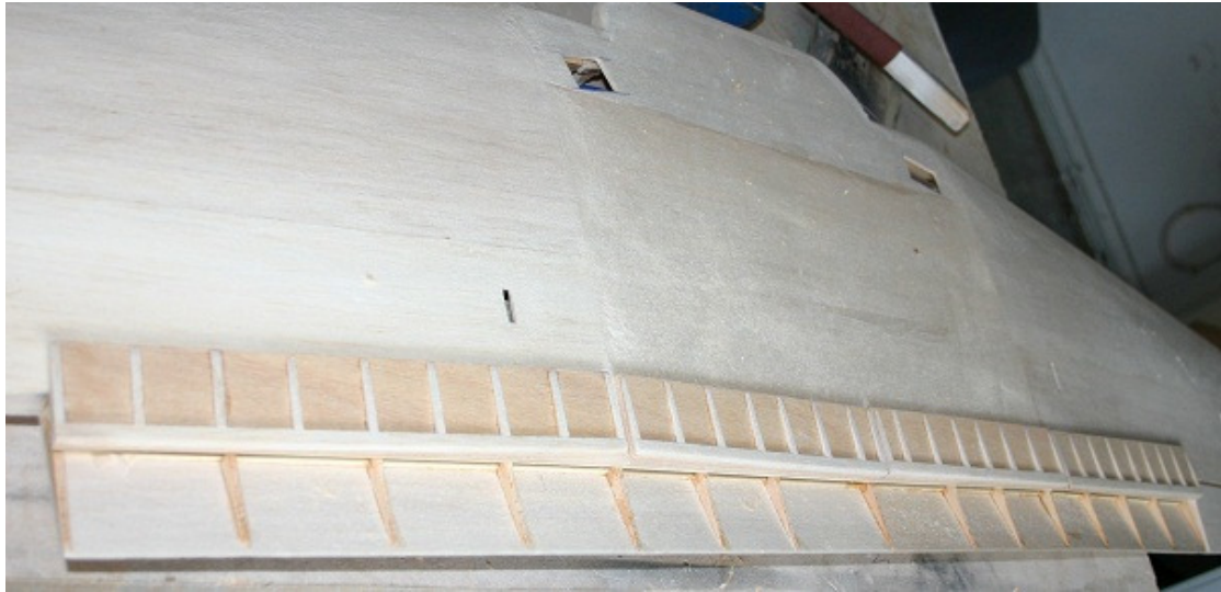
Flaps made up in 4 sections
