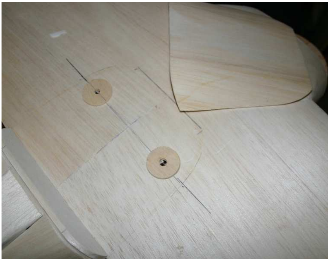
Wing fillet rolled from 3mm soft balsa
