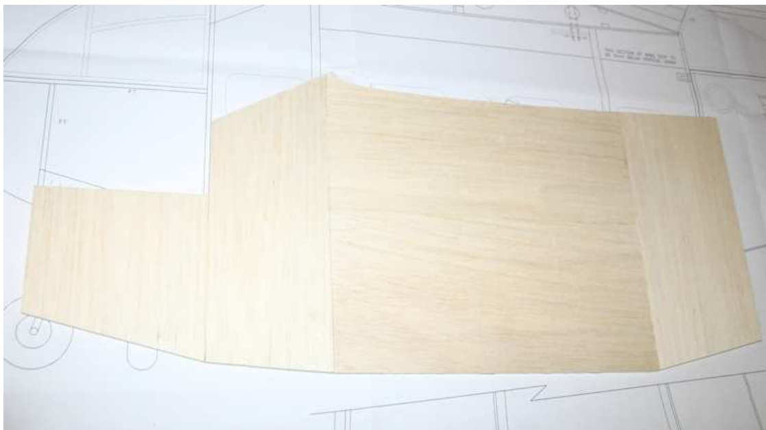
Fuselages side cut from pattern on plan-note grain direction
