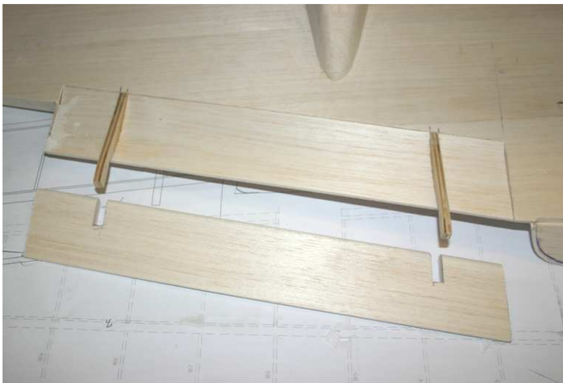
Flap made from solid balsa
