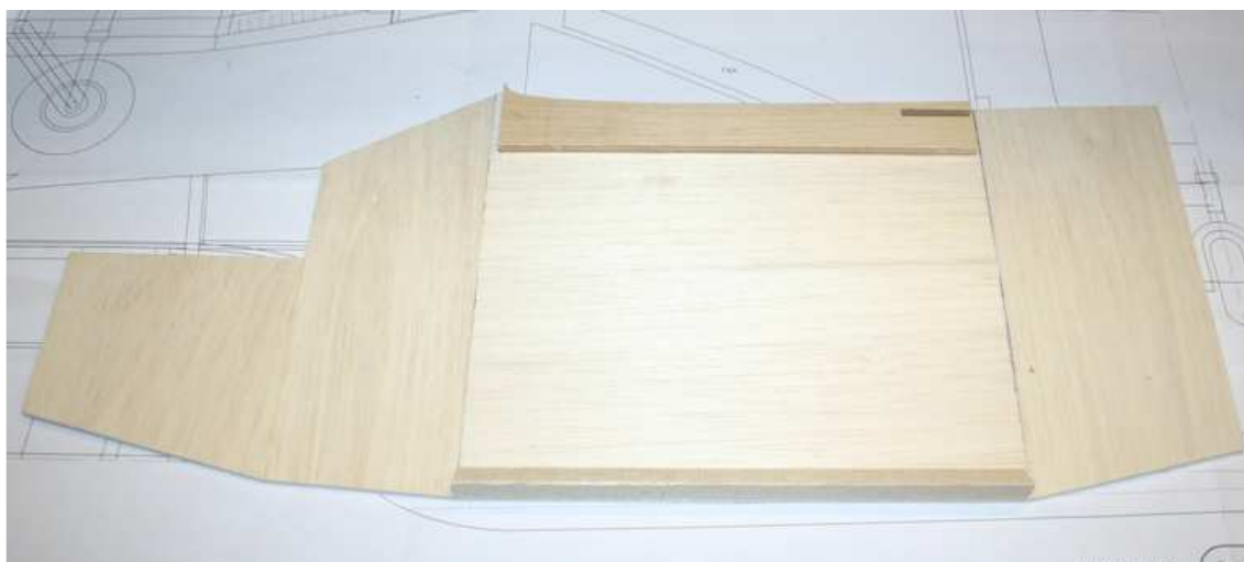
Fuselage side with wing doubler fitted and triangular edging
