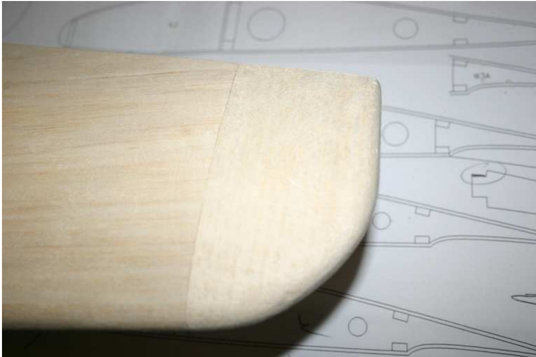
Wing tips made from solid balsa
