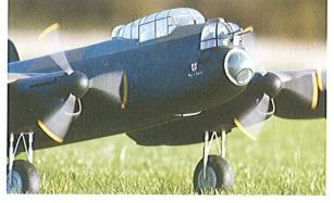
Speed 400s flat-out for any length of time will possibly damage them, so do consider cutting additional holes in the firewalls and, for the outer nacelle, a slot in the underside to allow cooling air to exhaust.
