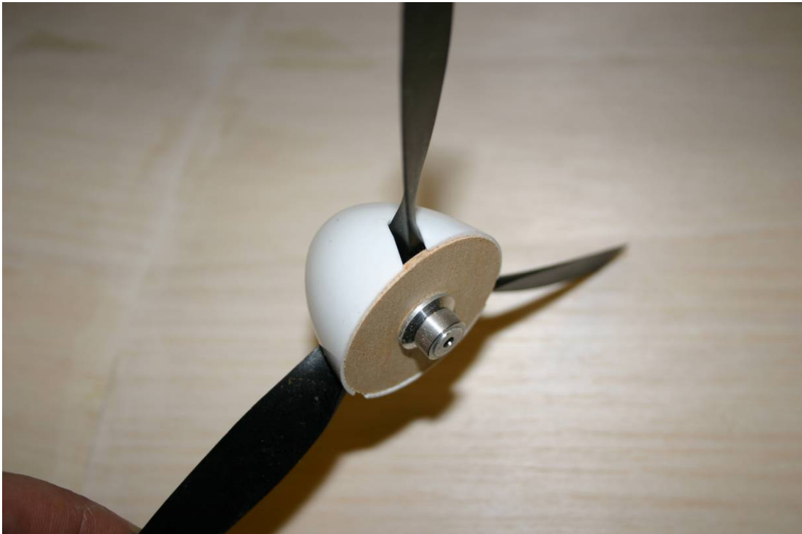
Prop used on the prototype 9"x7" cut down to 8" bought from Filtehook Models
