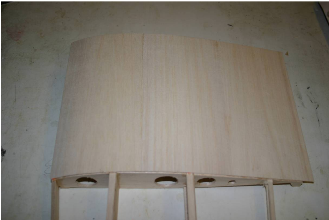
Outer & Inner panel joined and top sheet applied
