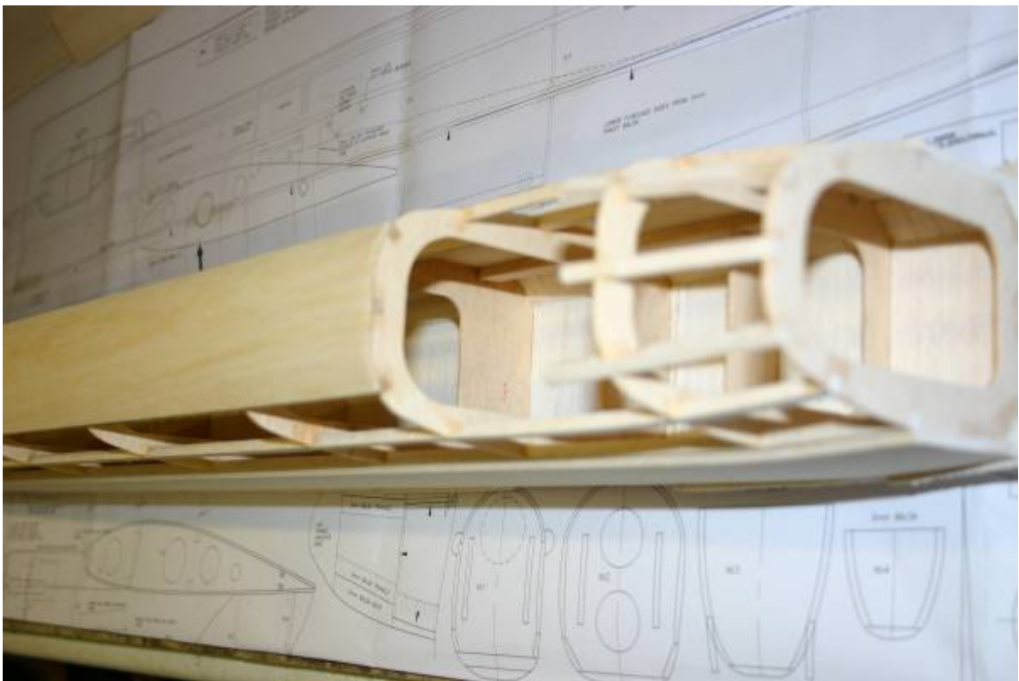
Sheet along the top first before sheeting the sides
